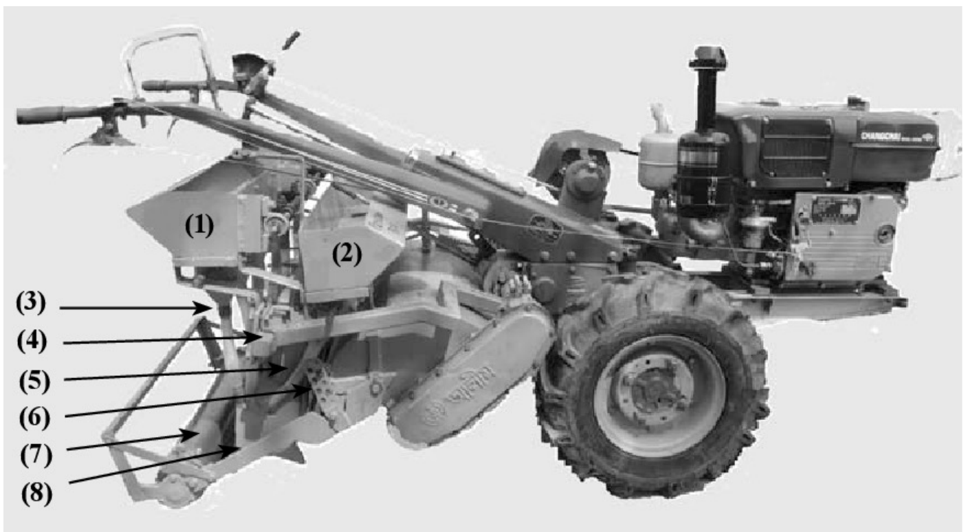
1: Seed box, 2: Fertilizer box, 3: Seed delivery tube, 4: Toolbar frame 5: Fertilizer delivery tube, 6: Depth controller, 7: Press roller, 8: Furrow opener
