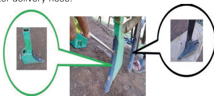
Furrow opener, the green one is furrow opener for fertilizer while the black one is for seed.
