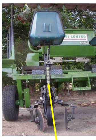
Photo 5. Spring device to control planting depth of the cassava stake.
