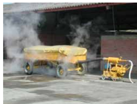
Photo 6. Steam sterilization of the substrate to avoid the presence of nematodes.
