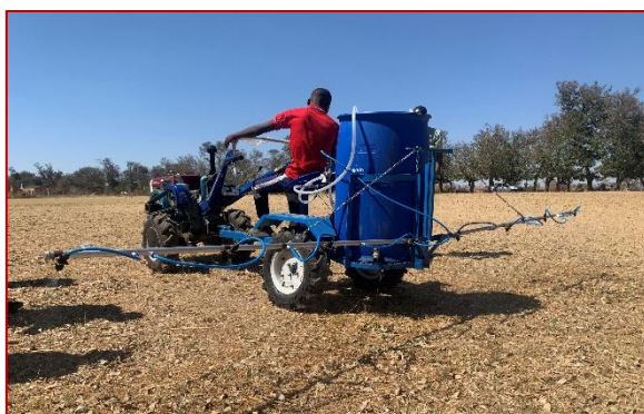
c) The boom sprayer (5 m, 200 l)
