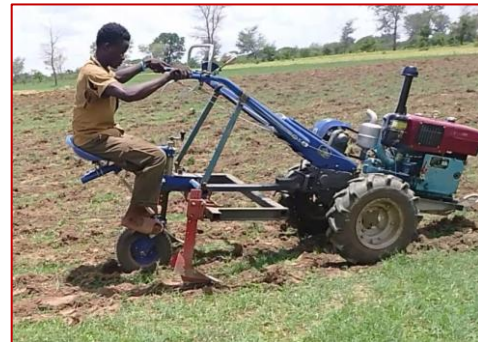
b) The double row-ripper in operation
