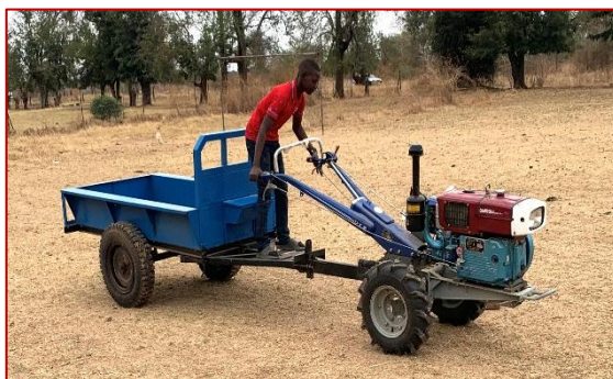
a) The trailer attached to a 2-wheel tractor
