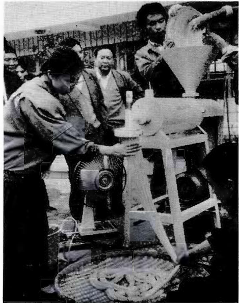
Making sweet potato noodles with a starch extruder in Sichuan Province, China.
