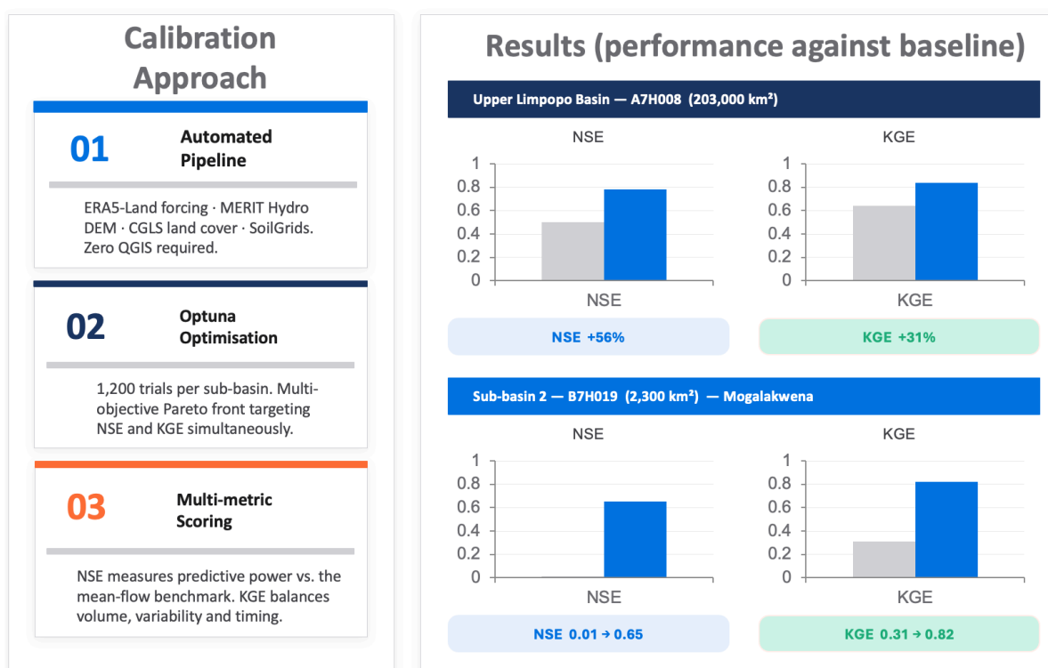
Figure 7. Calibration approach (left-hand panel) and calibration results (performance against baseline – right-hand panel). NSE = Nash-Sutcliffe Efficiency; KGE = Kling-Gupta Efficiency. Source: AI71 and IWMI (2026)
