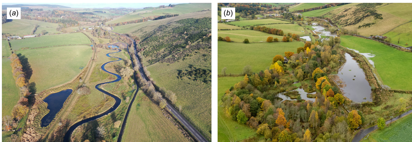
Fig. 3. (a) Re-meandering of a 3.5-km straightened stretch of the Eddleston Water, south-east Scotland; (b) Re-connecting the river and its floodplain. Figures reproduced by permission of Tweed Forum.
