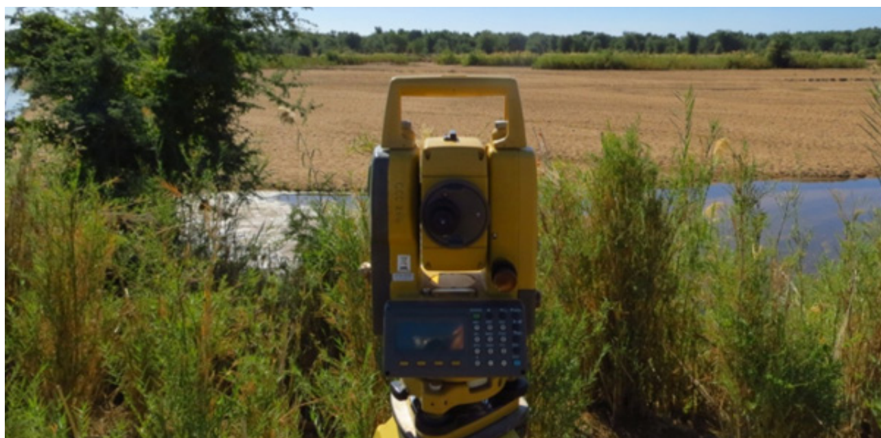
Total station measurement of cross-sectional dimensions to estimate river flow and stream morphology—the Limpopo River, Southern Africa ( photo : Bennie van der Waal).
