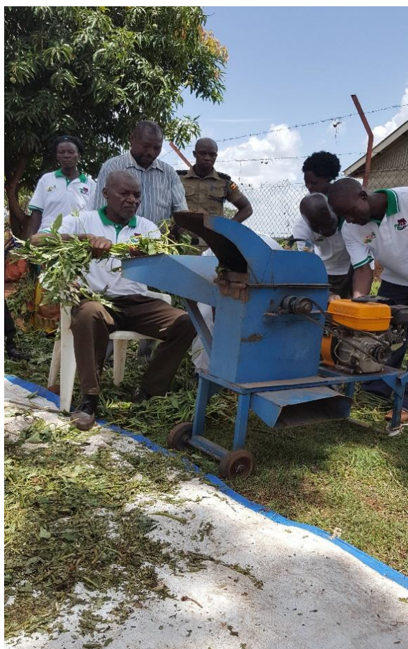
A farmer chopping sweetpotato vines using a motorized forage chopper
