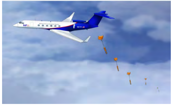
Figure 1.3-7: Left: Launching a weather balloon with instruments attached. Right: a storm monitoring aircraft releasing dropsondes to record atmospheric conditions within a storm. Sources: https://www.forbes.com/sites/marshallshepherd/2018/05/18/it-was-weather-balloon-georgia-not-a-bomb-5-questions-answered-about-them/ , https://scied.ucar.edu/learning-zone/atmosphere/dropsonde , accessed 10 Feb 2025.
