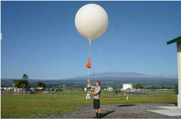
Figure 1.3-7: Left: Launching a weather balloon with instruments attached. Right: a storm monitoring aircraft releasing dropsondes to record atmospheric conditions within a storm. Sources: https://www.forbes.com/sites/marshallshepherd/2018/05/18/it-was-weather-balloon-georgia-not-a-bomb-5-questions-answered-about-them/ , https://scied.ucar.edu/learning-zone/atmosphere/dropsonde , accessed 10 Feb 2025.
