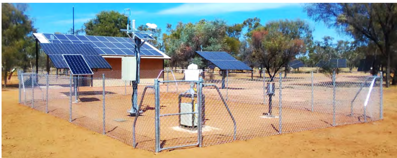
Figure 1.3-5: Traditional weather station site. This weather station includes a rain gauge, temperature gauge, relative humidity, barometer, anemometers, pyranometers, and pyrliometer with solar panels to power the sun tracker and some sensors. Source: https://www.essearch.com/compact-weather-sensors-and-traditional-weather-sensors/ , accessed 10 Feb 2025.
