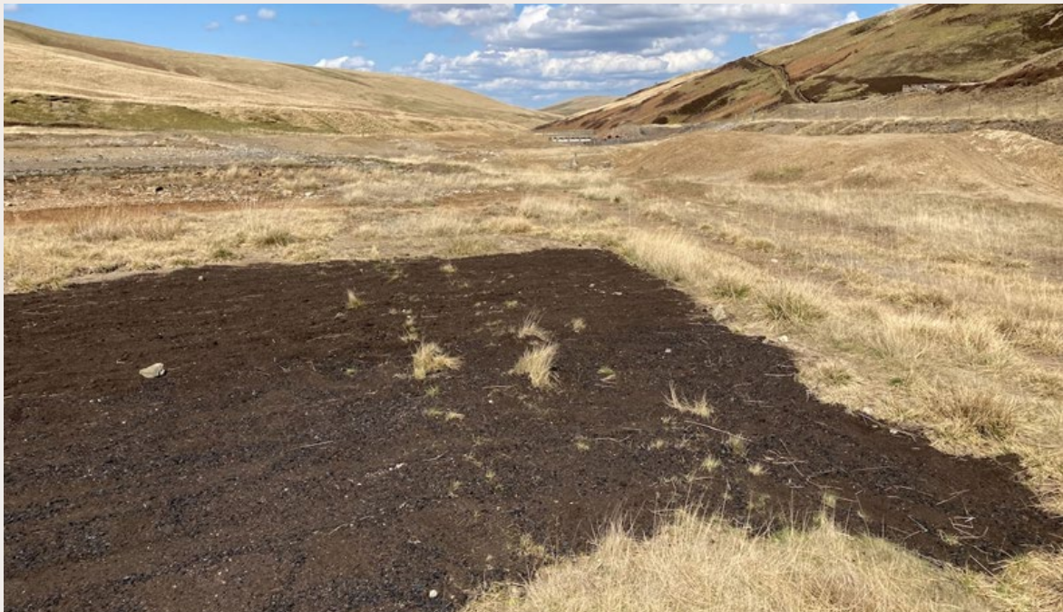
FIGURE 9. Application of biochar and compost to a barren area of eroding lead mine tailings during CERESIS Project phytostabilization field trials in Scotland.
