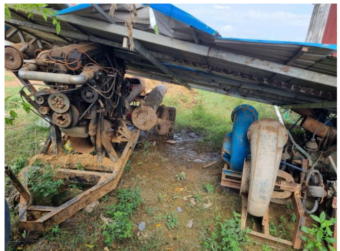
Figure 4. Large diesel pumping machines, modified from trucks, stationed and unused during flood seasons from August to October
