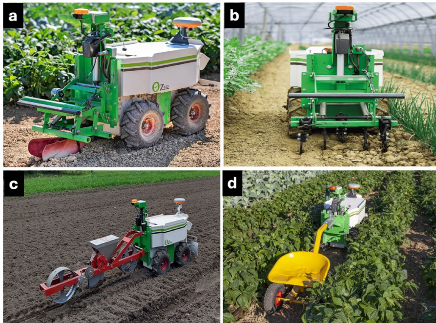
Fig. 3 Oz multi-purpose robot. a furrowing, b hoeing, c sowing, d transporting
