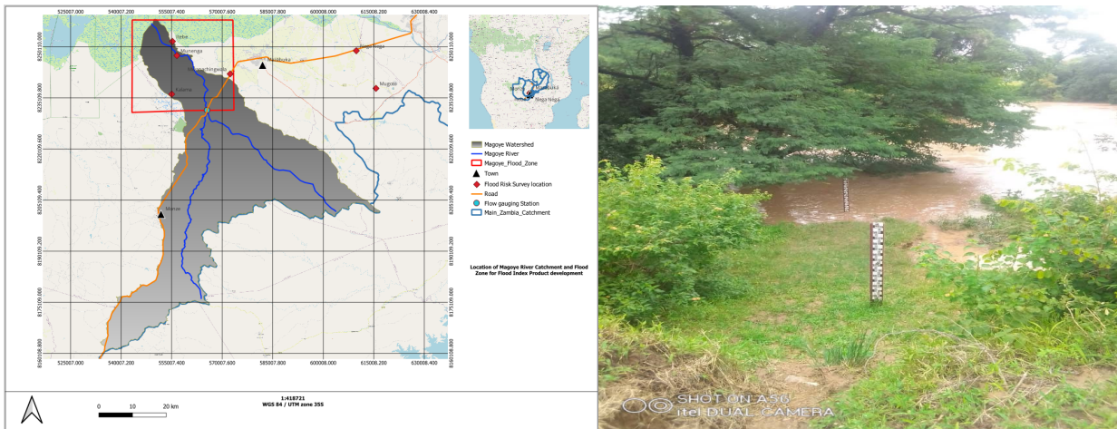
Figure 1. Left: Magoye River Catchment, red rectangle indicates Flood Zone in the downstream of the river. Right: location gauging station with flooding building up for flood event in 2023: Source Authors.
