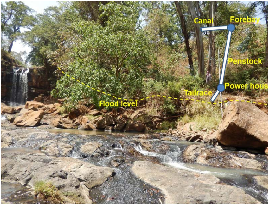
Figure 12. Schematic view (above), panoramic view for diversion site (middle), and penstock (and powerhouse) site (below) of the proposed Engrin MHP site, Amhara region, Ethiopia.
