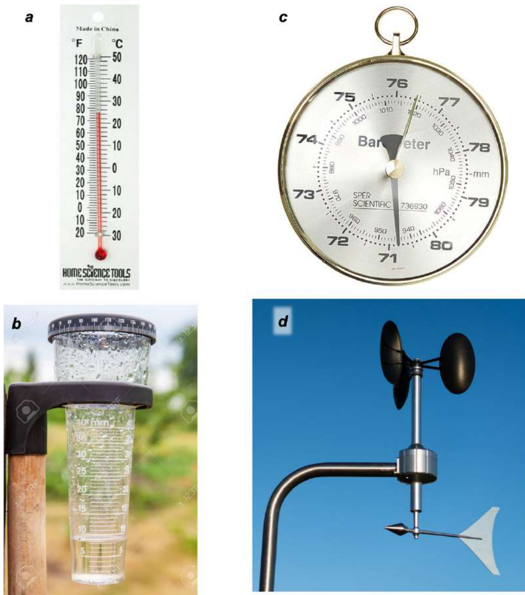
Figure 1.3-4. Common manual meteorological measurement instruments: mercury thermometer (a), rain gauge (b), barometer (c), anemometer (d). Sources:
