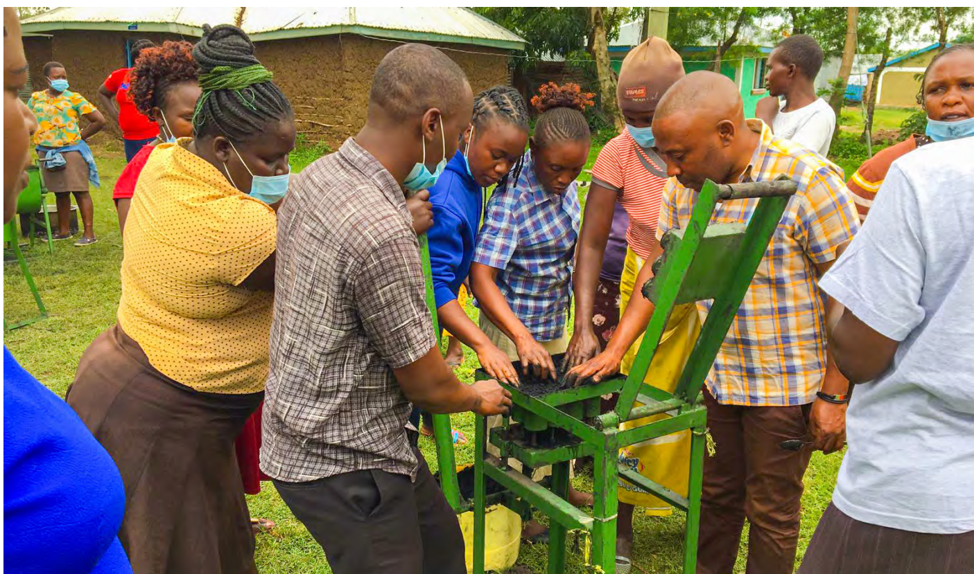
Women group in Kisumu, Kenya learning how to operate a manual briquette press ( Photo Credit: James Kinyua Gitau).
