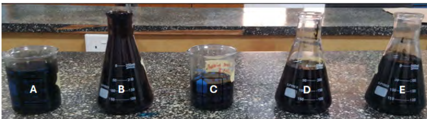
Figure 7: Bio-oil from various feedstocks: a) pruned wood (day 1), b) pruned wood (day 2), c) pruned wood (day 3), d) palm kernel shells, and e) sawdust.
