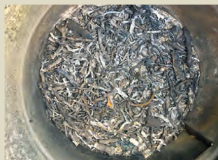
Figure 2: The full-drum kiln: a) loaded with biomass, b) during carbonization and c) char produced. Photo Credit: James Kinyua Gitau
