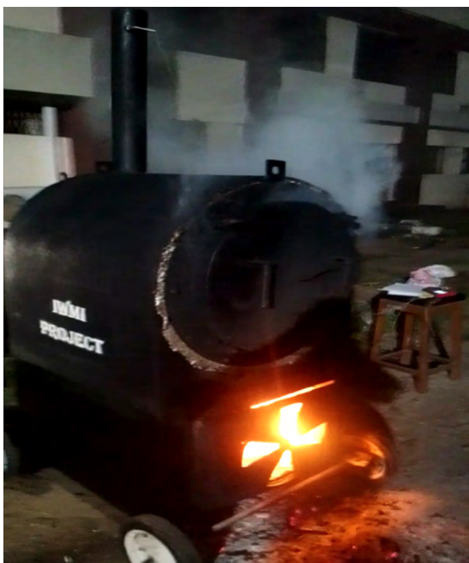
Figure 8: Troubleshooting the carbonisation equipment: a) leakages at the front cover and b) no leakages after a fire-resistant material is installed.
