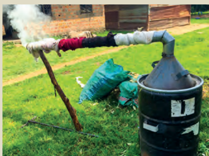
Figure 2: The full-drum kiln: a) loaded with biomass, b) during carbonization and c) char produced. Photo Credit: James Kinyua Gitau
