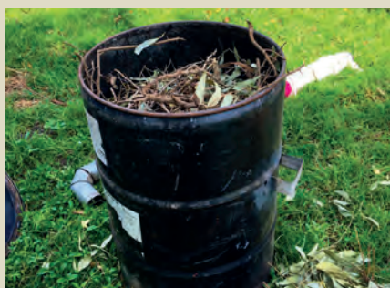
Figure 2: The full-drum kiln: a) loaded with biomass, b) during carbonization and c) char produced. Photo Credit: James Kinyua Gitau
