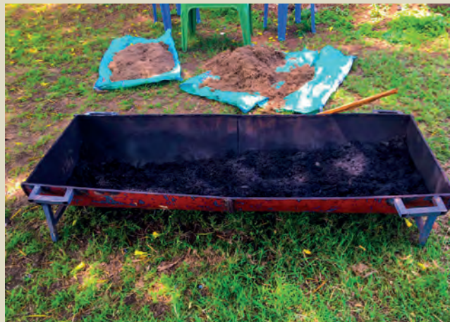
Figure 1: The Open Half-Drum Kiln: a) Women carbonizing in a half drum kiln and b) char produced. Photo Credit: James Kinyua Gitau
