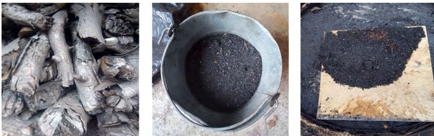
Figure 6: Biochar yield from various feedstocks: a) Charred wood logs, b) bio-char produced from palm kernel shells and c) bio-char from sawdust.
