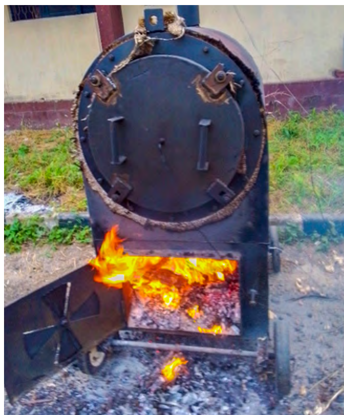
Figure 8: Troubleshooting the carbonisation equipment: a) leakages at the front cover and b) no leakages after a fire-resistant material is installed.
