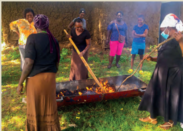
Figure 1: The Open Half-Drum Kiln: a) Women carbonizing in a half drum kiln and b) char produced. Photo Credit: James Kinyua Gitau
