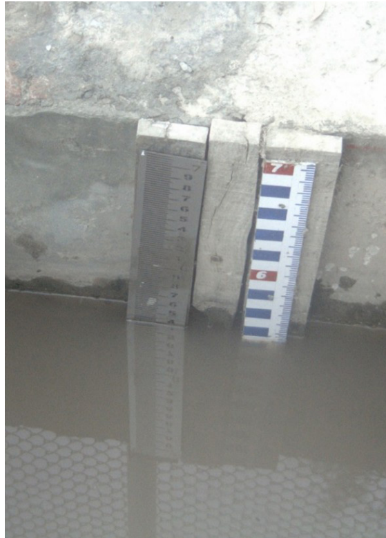
Figure 10. Stainless Steel Staff Gauge and ordinary painted gauge installed in a stilling well at the Lower Bari Doab Canal. (photo: Muhammad Tousif Bhatti/IWMI)
