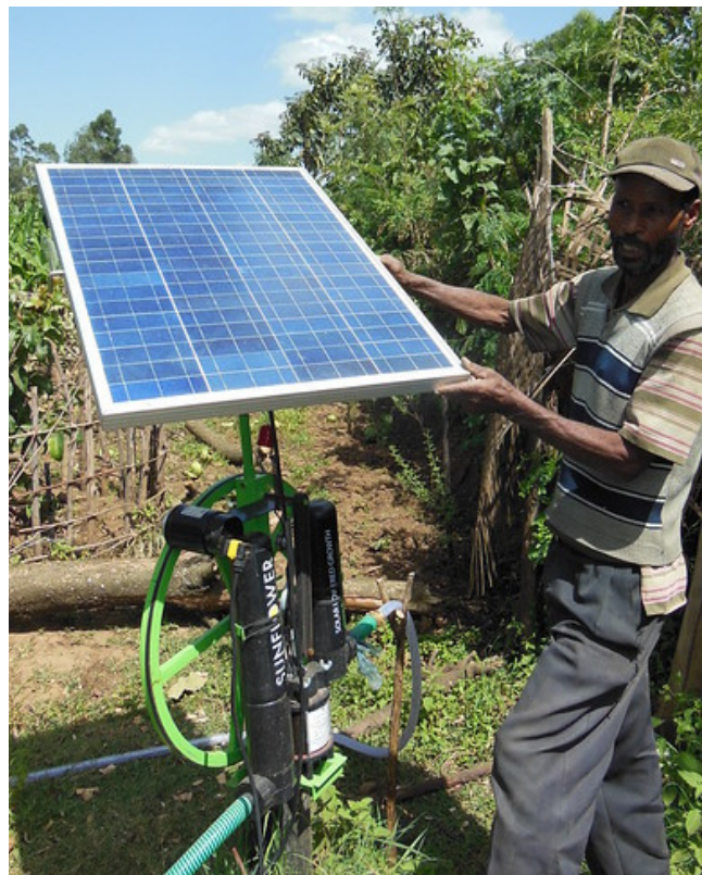
A farmer in Lemo worda with his newly installed solar irrigation pump (Photo: Petra Schmitter/IWMI)
