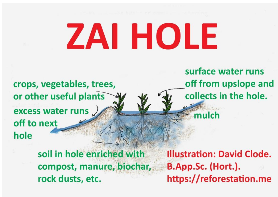
Fig 6: Zai/Halfmoon technique in Land rehabilitation
