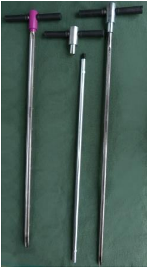
Figure 1. Left: Different types of Pürckhauer soil augers: Large-diameter auger with fixed head (left); auger with detachable head (middle); small-diameter auger (right) Note the cross bar is removed when hammering the auger into the soil.
