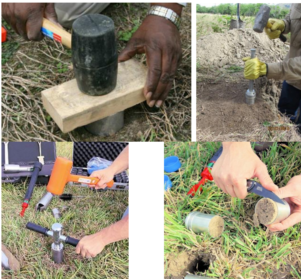
Figure 12. Upper left: Soil cylinder being hammered into the soil from the surface with a mallet and a piece of wood to cushion the mallet strikes. Upper right: Soil cylinder set in a gadget with a long handle to insert vertically into the soil. Lower left: Soil cylinder set in a gadget with a short handle and cross bar, hammered into the soil. Lower right: Soil cylinder recovered from the soil and the excess soil being cut off with a knife along the lower edge of the cylinder
