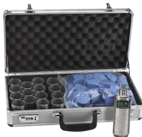
Figure 6. Left: Steel soil core samplers of different dimensions with a sharpened edge to cut into the soil. Right: padded suitcase to transport soil cores, blue lids for the cores and a sampling tool (front) into which cores are inserted and pushed into the soil
