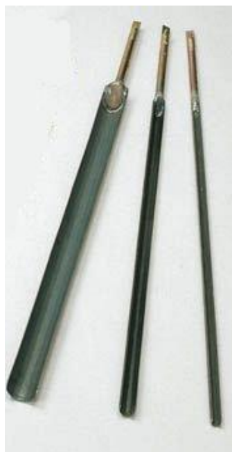
Figure 4. Examples of detachable augers with different diameters and openings
