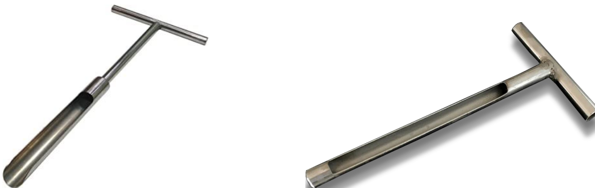
Figure 2. Left: Soil auger with an open tip. Right: Soil auger with closed tip. Both with a fixed handlebar to push the auger manually into the soil
