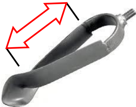
Figure 5. Detachable tip of an Edelman auger
