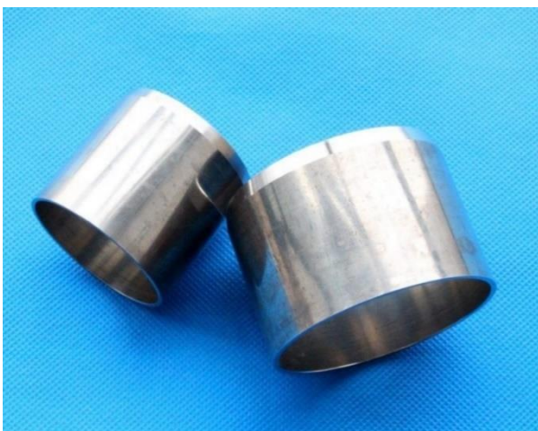
Figure 6. Left: Steel soil core samplers of different dimensions with a sharpened edge to cut into the soil. Right: padded suitcase to transport soil cores, blue lids for the cores and a sampling tool (front) into which cores are inserted and pushed into the soil
